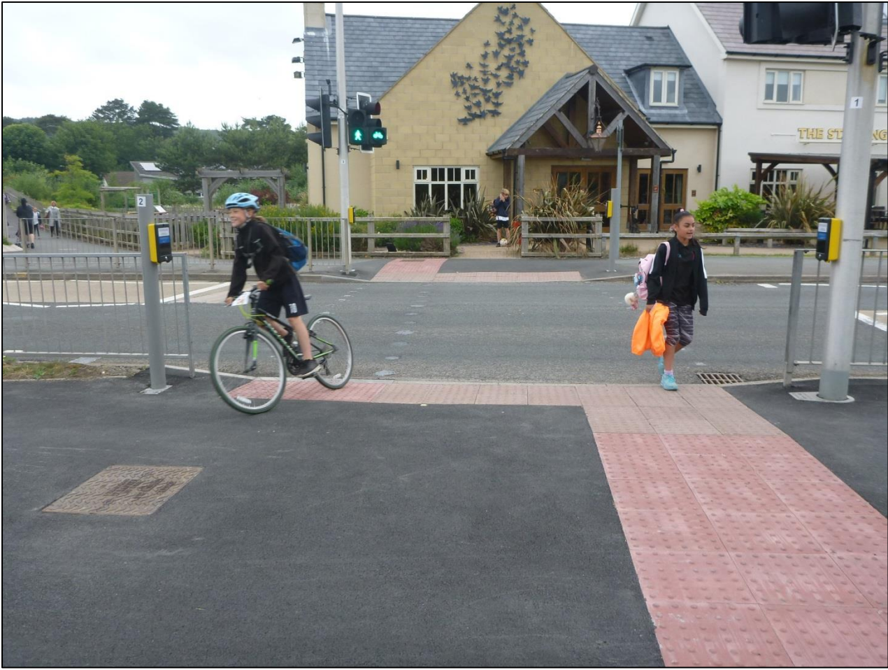
Below: Crossing upgraded to a Toucan for cyclists to now use as well as pedestrians:
