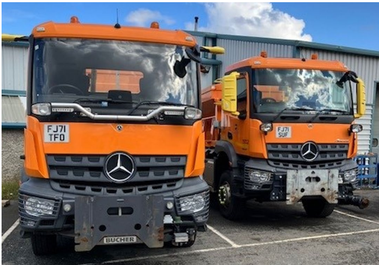
Figure 16 – On the left is a Mercedes 6x4 with Bucher gritter body. On the right is a Mercedes 4x4 fitted with a Bucher Electra lithium battery-powered road gritter. It replaces traditional hydraulics with high-efficiency onboard battery packs, delivering zero emissions, reduced salt waste, and up to 20 hours of operation per charge.
