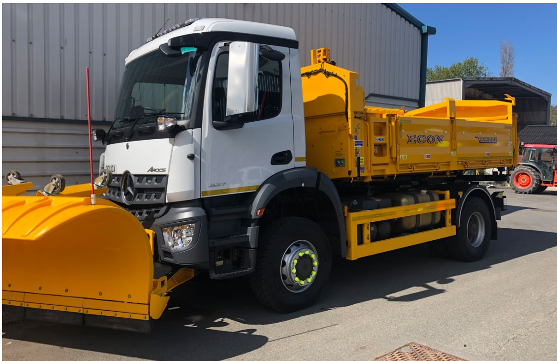
Figure 15 – Mercedes 4x4 fitted with an Econ Unibody, a specialized 6m 3 , 18-tonne multi-purpose road maintenance and winter service vehicle. It combines gritters, de-icers, and insulated tippers into a single chassis to handle year-round tasks like salting and road patching.
