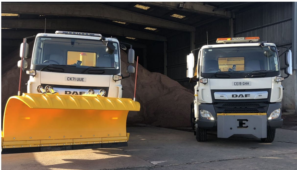
Figure 3 – DAF unibody gritters. Used for Highways surface dressing in the summer months, snow ploughing and gritting duties in the winter months.
