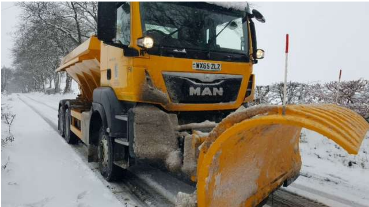
Figure 5 – Designated 26t tonne MAN gritter in action.
