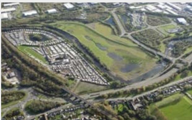
*Completed in 2014, this £6.9 million scheme made space for water by forming new earth embankments creating an area to hold flood water from the River Tawe and its tributaries during flood events. As well as raised embankments the scheme creates more space for water by setting back the flood defences at the top end of the river and taking out three redundant bridges to allow more water to pass.*
